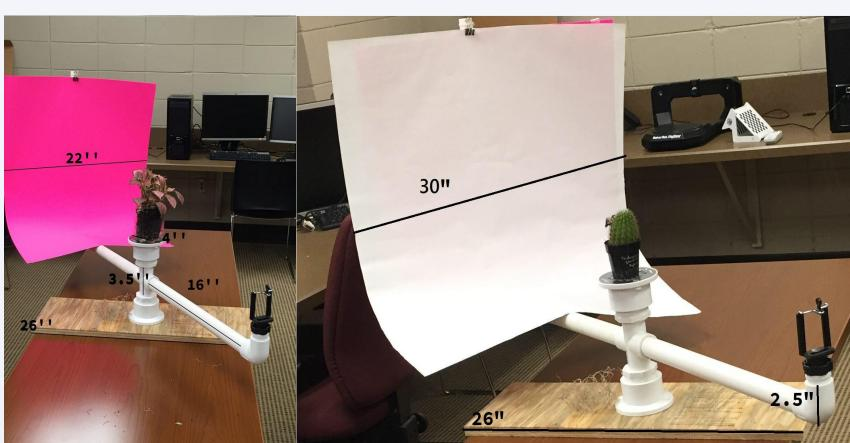
We created a rig that holds a plant static relative to a rotating camera and backdrop. We used two different background colors: white and hot
